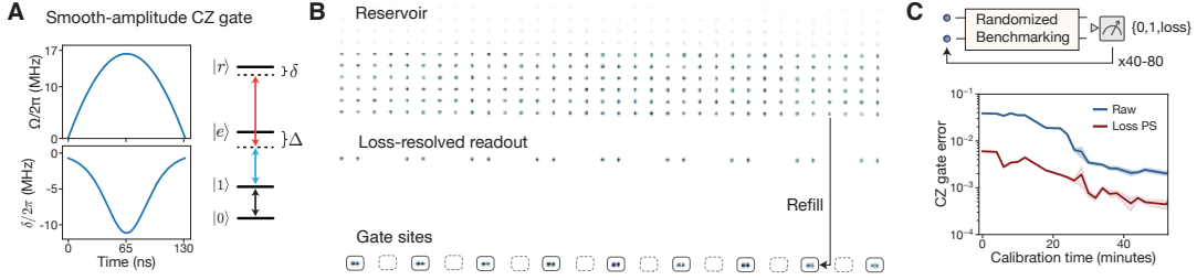
Figure 8.1: CZ entangling gates in a neutral atom processor with fast cycle rates. (A) Rydberg gate realized through a smooth-amplitude gate pulse at roughly \Omega = 2\pi \times 17 MHz peak Rabi frequency, with a detuning profile \delta(t) . Two-photon excitation scheme consists of transitions at 420 nm and 1015 nm, exciting from qubit state |1\rangle to the Rydberg state |r\rangle = 53S_{1/2}, m_J = -1/2 through the intermediate state manifold |e\rangle = 6P_{3/2} with intermediate state detuning \Delta = 2\pi \times 7.8 GHz. (B) Images of the atoms separated into processor zones, with gate sites used for benchmarking and high-fidelity quantum circuits, and state-selective readout to perform loss detection. Fast calibration of CZ gates is enabled by qubit reuse and refilling lost atoms from a large atom reservoir. (C) Randomized benchmarking is performed over 40-80 repetitions, with a 20-30 Hz cycle rate. Example calibration of the CZ gate from starting parameters near the theoretical prediction, showing both raw and loss-postselected CZ error. Each point corresponds to the fitted maximum of a parabola scan over one of the gate parameters, with error bars given by the shaded region.
